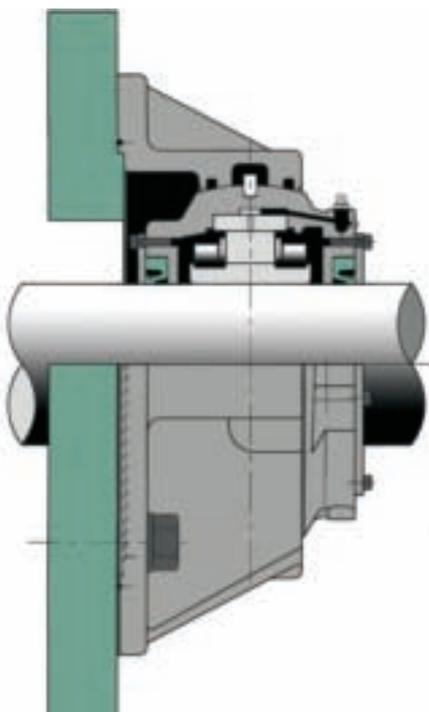
Flange unit with bulkhead seal
