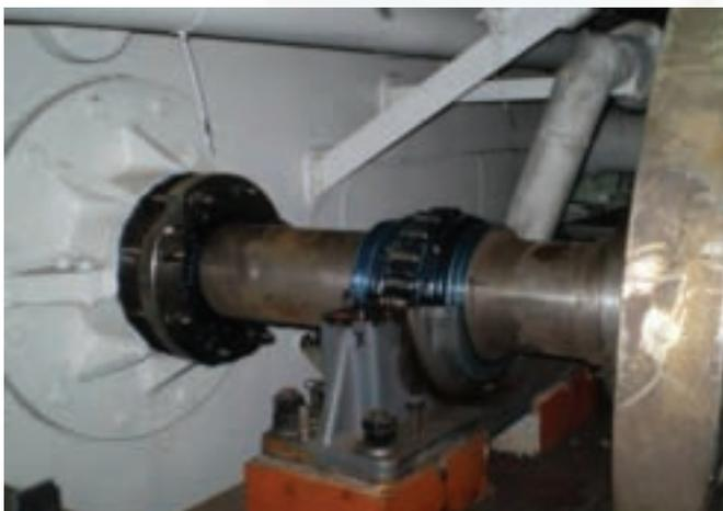
Cooper bearing on a marine generator drive during inspection
