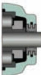
Machined aluminium bodied triple labyrinth seal for high speed and general applications. ATL supplied as standard sealing arrangement in USA and Canada. ATL HT and ATL LT are fitted with O rings of different materials.
