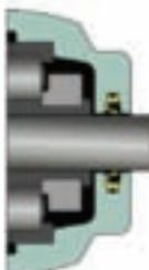
Suitable for wet but not submerged conditions.
